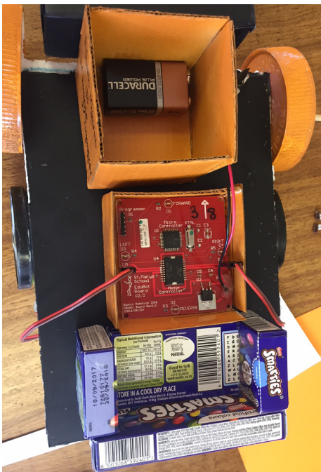
Circuit board and battery in situ on a robot
